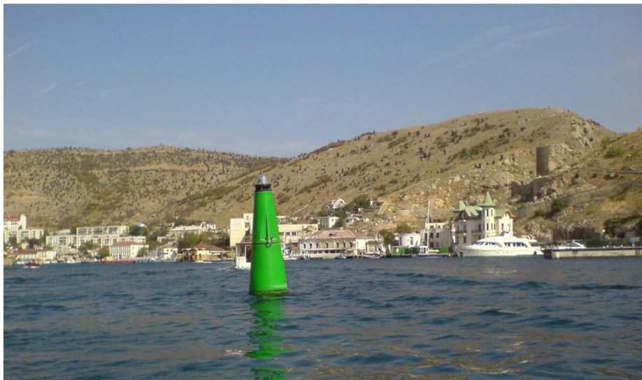
Ballast is attached to lower part that ensures stability of the buoy taking into account possible currents and wind load.
